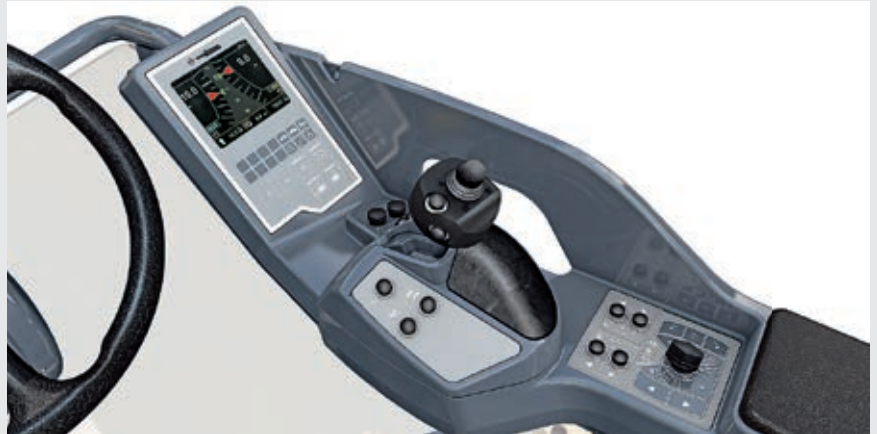
Machine height adjustment integrated in the multi-functional armrest
